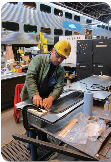
A new seal is placed around a window as part of the Amerail railcar rehab at the 49th St. Shops.
