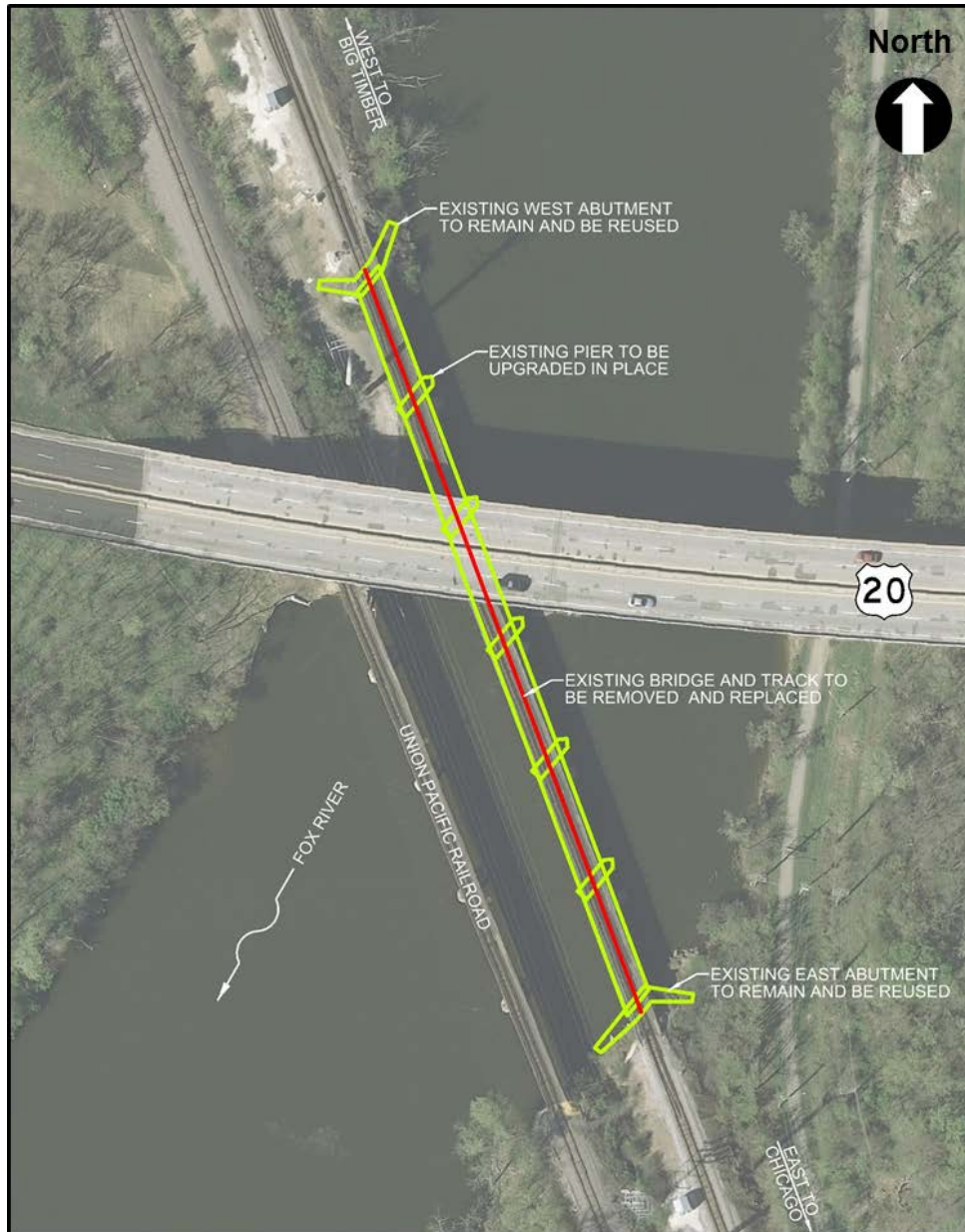
Figure 2-2: Components of Alternative 2 – Construct a New Single-Track Bridge on the Existing Alignment
