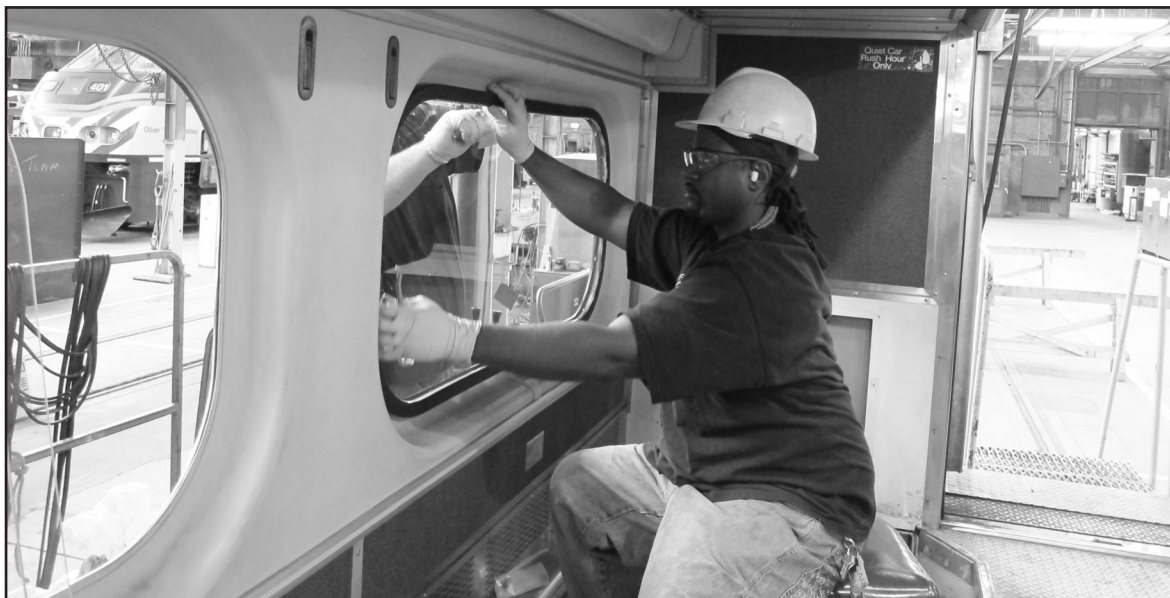
Carman Bryant Howse replaces a window on an Amerail passenger car at Metra's 49th St. Shop, where the Amerail rehab program is based.
