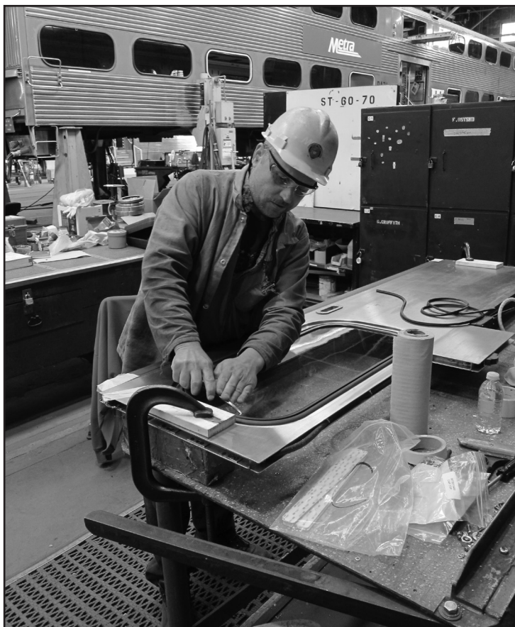
Carman Frank Osysko replaces a window in a door from one of the Amerail cars being rehabbed by Metra workers at the 49th St. Shop along the Rock Island Line.
