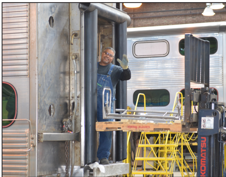
Glendon Griffith, a veteran carman in Metra's program to rehabilitate passenger cars, unloads seat frames for installation in one of the cars being worked on.
