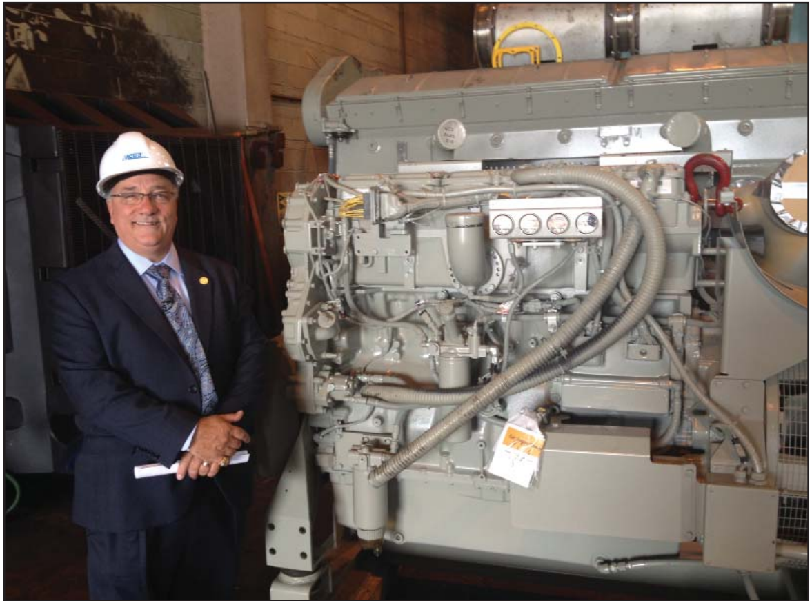
Metra Executive Director/CEO Don Orseno stands next to one of the new genset diesel engines that is being installed into Metra's fleet of 27 MP36 locomotives to power the onboard systems and improve passenger comfort and boost the locomotives' reliability.
