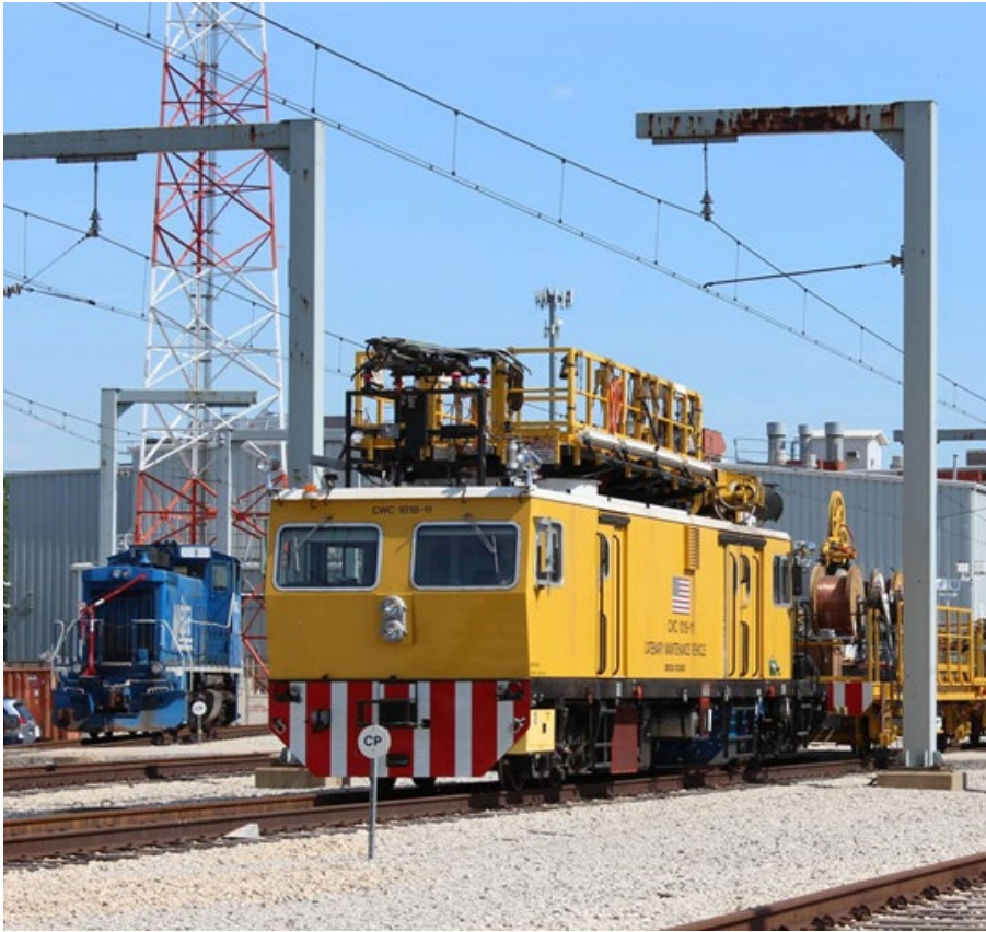
Metra Electric District catenary maintenance vehicle
